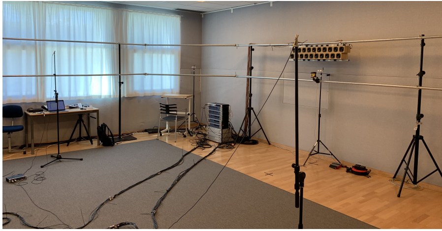
Figure A.1: Picture of the test setup for the recordings of pressure in the acoustical bright and dark sound zone for CT computations.
